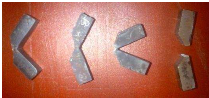
Fig. 4 Charpy Impact Test Samples after Fracture
