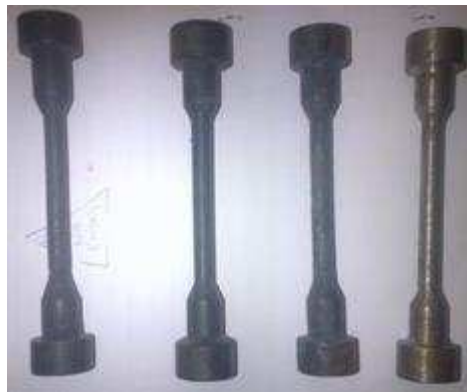
Fig. 2 Annealed Samples before undergoing Tensile Test.
