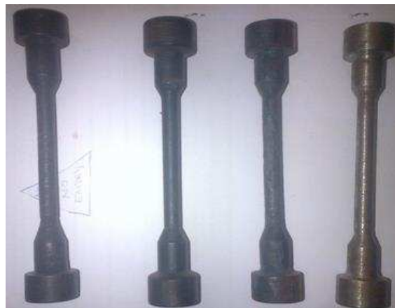
Fig. 1 Annealed Tensile Test Specimen
