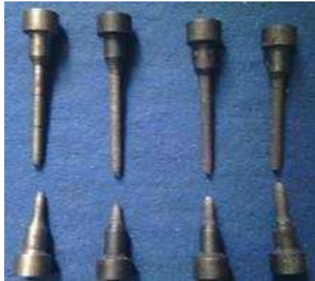
Fig. 3 Annealed Samples after undergoing Tensile Test
