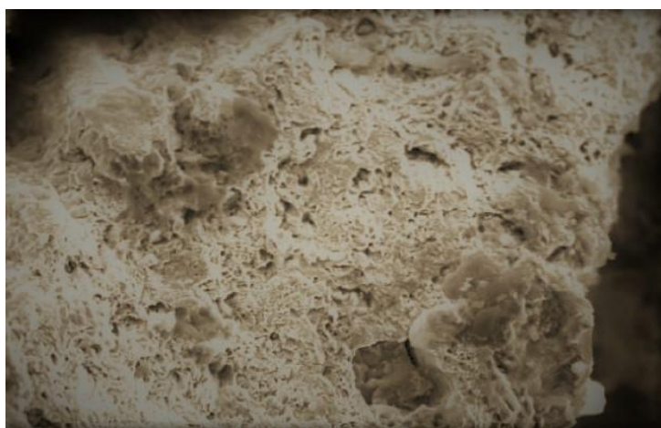
Figure 5: SEM at 25 kv Fractograph at the Neck Portion Showing Brittle Fracture at X200 Magnification Factor
