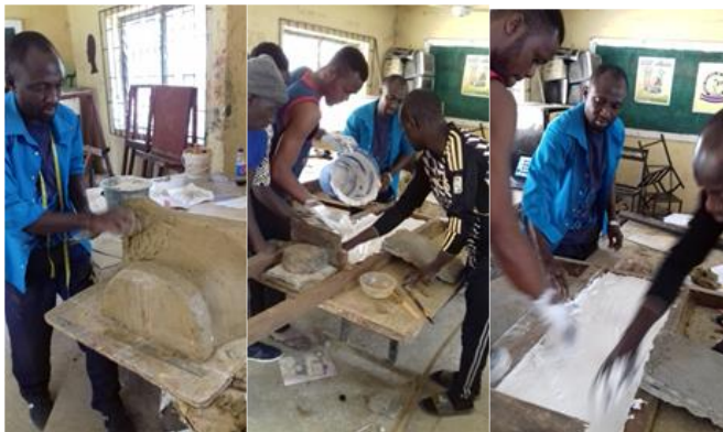
Figure 5. (a) Modeling; (b) Mould making; (c) Casting (Adebawale, 2020)
