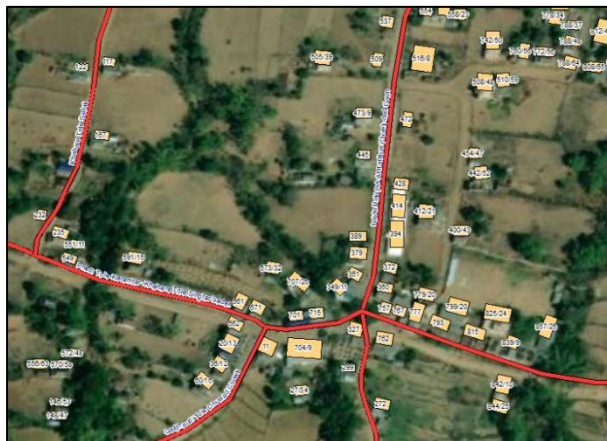
Fig 9: Metric house ID within building footprint
