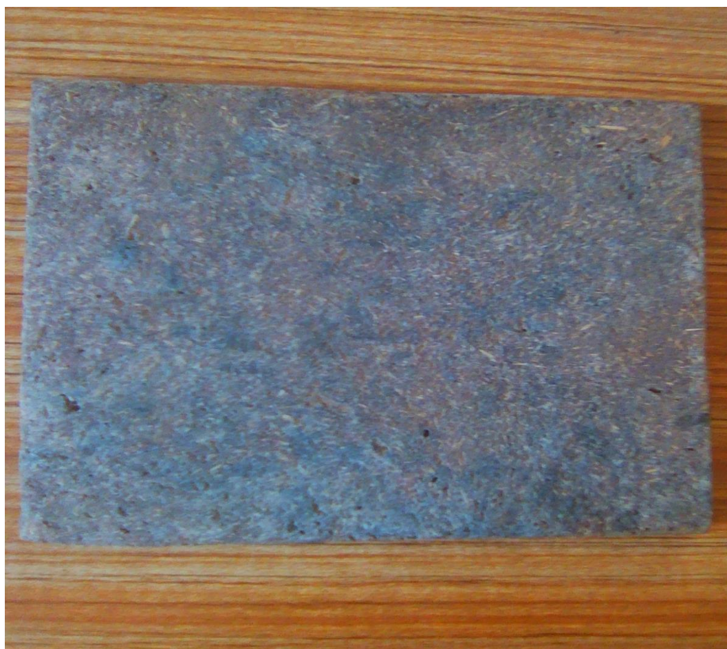
Plate I: Reproduced piliostigma thonningii ceiling board experimental sample
