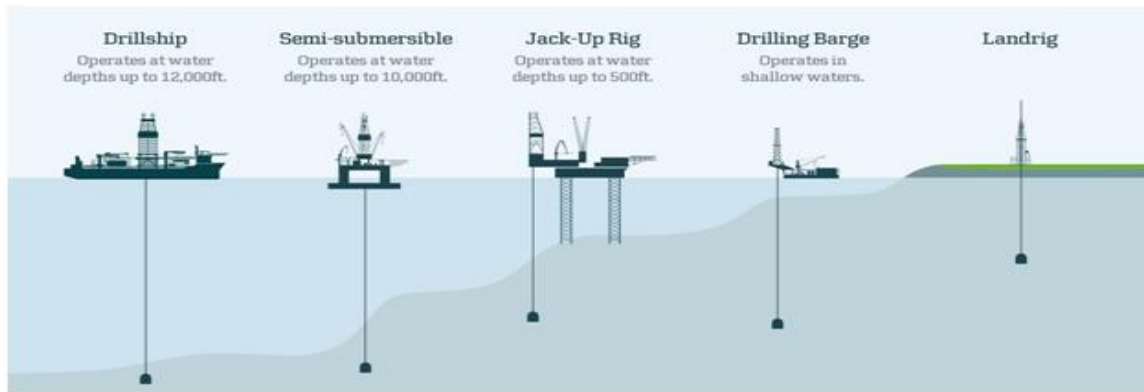
Fig.5: Diagram of different types of offshore drilling rigs.
