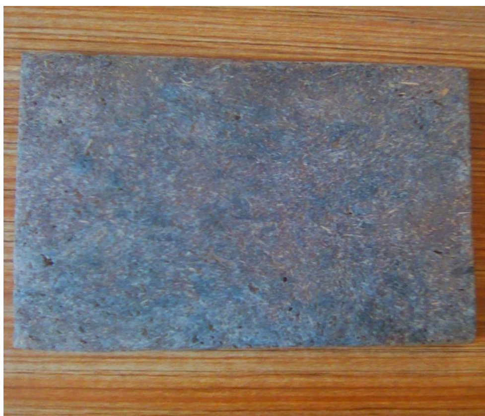
Plate I: Reproduced piliostigma thonningii ceiling board experimental sample
