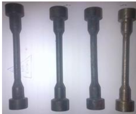
Fig. 2 Annealed Samples before undergoing Tensile Test.
