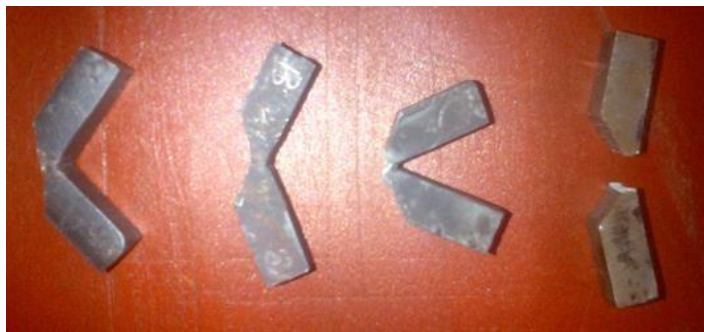
Fig. 4 Charpy Impact Test Samples after Fracture
