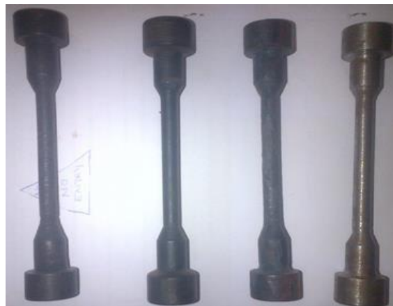
Fig. 1 Annealed Tensile Test Specimen
