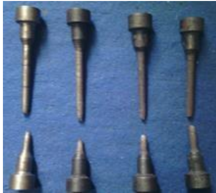
Fig. 3 Annealed Samples after undergoing Tensile Test
