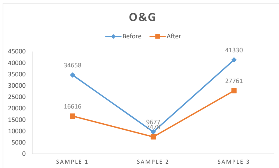
Fig 4: Removal of oil & grease using hydrochloric acid from waste coolant effluent sample
