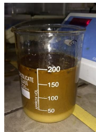
Fig 2: oil recovery after treatment from one litre of sample
