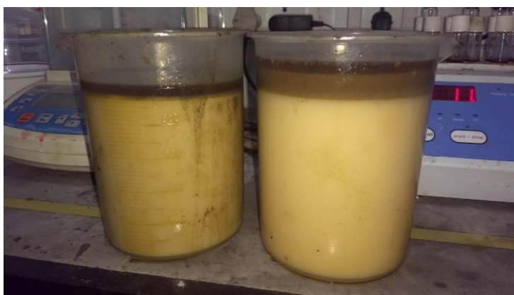
Fig 1: oil layer separation before treatment (Left) and after treatment (Right)
