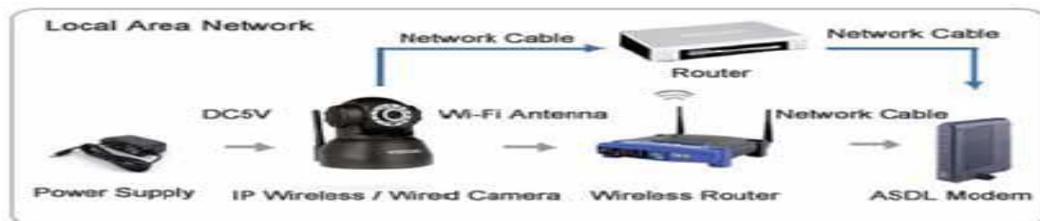
Figure 7: Connection Via A Router
