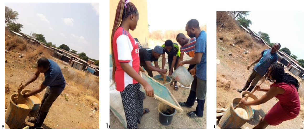
Fig. 2(a); (b) & (c.) Stirring of clay to soften solid particles
