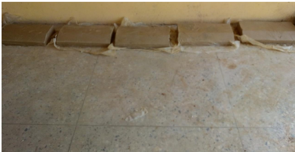
Fig. 6. Drying of clay-kerbs
