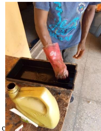
Fig. 5(c) Application of lubricant inside the mould
