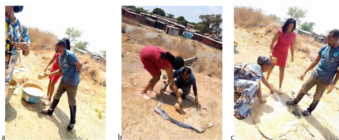
Fig. 4(a); (b) & (c). Preparation of clay slip to form clay ball
