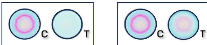
Fig.1 (a) no formaldehyde contamination; (b) Contaminated with formaldehyde less than 100 ppm.
