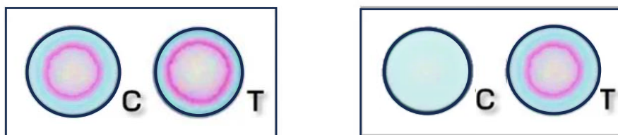
Fig.2 (a) Contaminated with formaldehyde more than 100 ppm.; (b) the test kit is unavailable.
