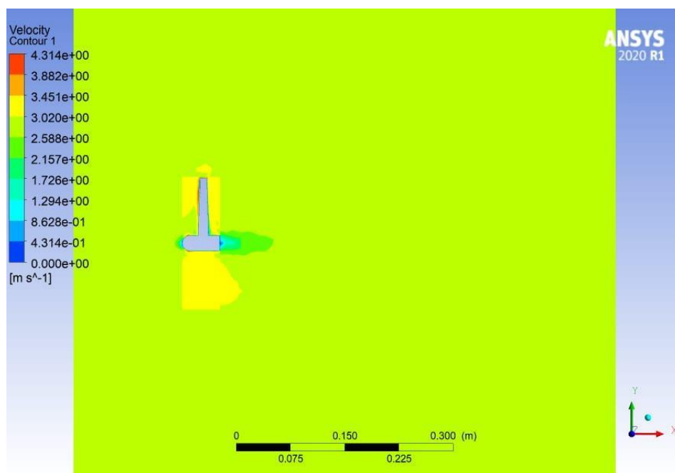
Fig. 10. Velocity field for the open-turbine configuration.
