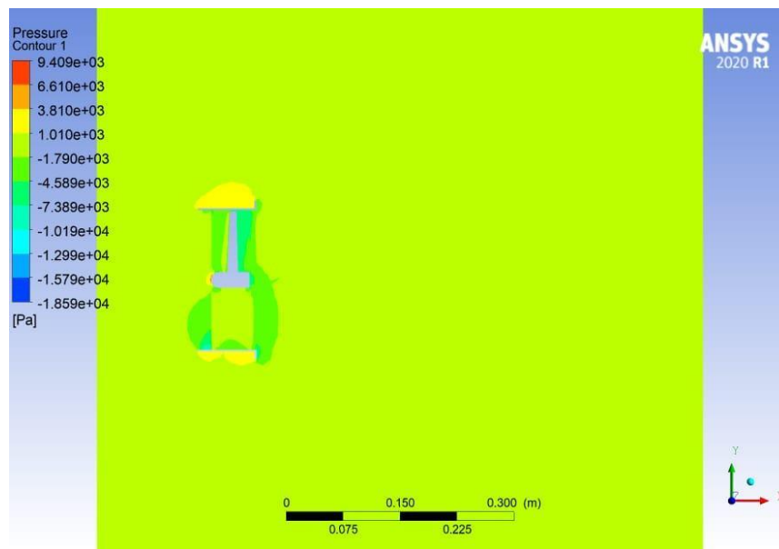
Fig. 8. Pressure contour for the short-expansion flanged diffuser.
